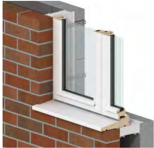
In check installation detail
